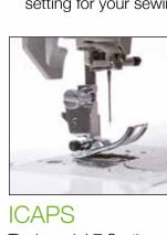
The Innov-is V7 Continuous Automatic Pressure System (ICAPS), continuously detects fabric thickness whilst you sew and automatically adjusts the foot pressure to give superior even stitch quality when stitching over differing fabric thicknesses. This is especially useful for free motion embroidery and ensures super-smooth constant stitching throughout
