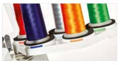
Thread stand with LED guide lights Multi-coloured LED lights help to show the position of broken threads, the position when a thread needs changing and the position thread for each colour used.
